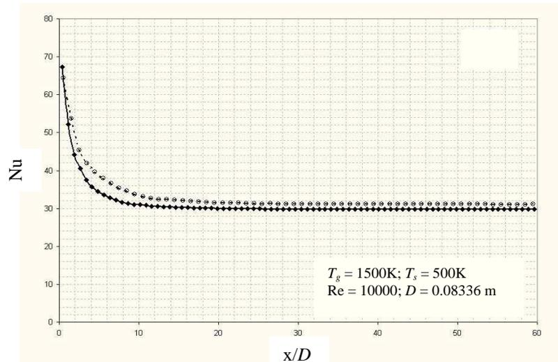
Figure 8. Local convective Nusselt numbers for pure convection and combined radiation-convection heat transfer. Gas mixture 2.
