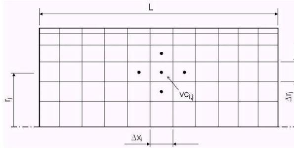
Figure 2. Surface and volume zones in the interior of a circular tube.
